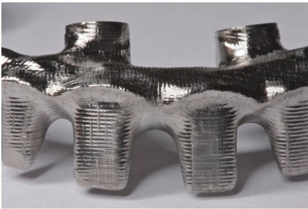
**Figure 2** CAD/CAM Titanium framework before finishing the margins.
